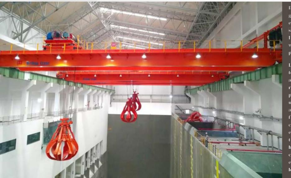
Double girder overhead crane for garbage is one of the green and environmentally friendly industry specific cranes developed by Weihua. It has served Chongqing Sanfeng waste incineration power generation project.
