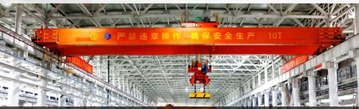
The intelligent unmanned crane independently developed by Weihua Group for the construction industry is customized and developed for the prefabricated construction industry. In 2021, Weihua provided Guangxi Construction Engineering with a fully automatic electromagnetic double girder overhead crane with carrier-beam.
