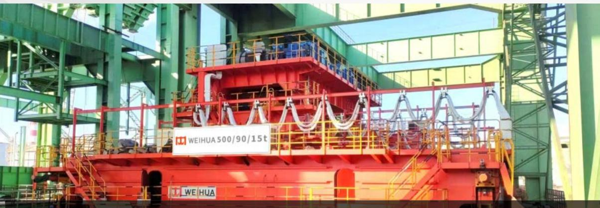
In 2022, four girder six rail metallurgical crane with the largest tonnage of 500t independently developed by Weihua Group serves Tangshan Ganglu Iron and Steel Co., Ltd.
